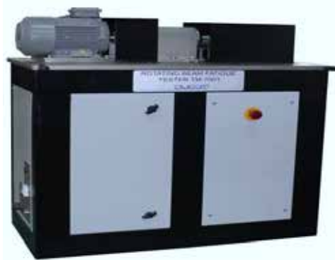
Figure 3.44 : Rotating Beam Fatigue Tester
